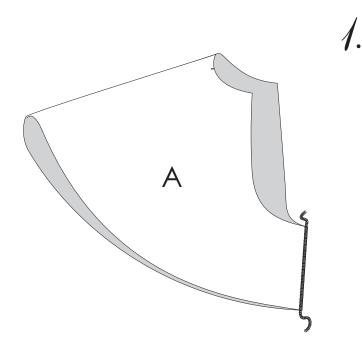
With right sides together overlock stitch front inseam to back inseam.
