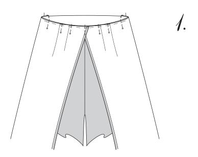
Pin straps to waist of shorts. Match center front strap notches to front seam of shorts. Straps will overlap 3 cm. Align edge of strap at side waist to notch. Baste straps to shorts within seam allowance.
