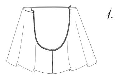
With right sides together overlock stitch the crotch seam matching center fronts and center backs.
