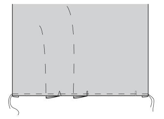
$\overrightarrow{J}. \quad \begin{array}{l} \text{Baste turned edges and pleats} \\ \text{in place within the seam allow-} \\ \text{ance.} \end{array}$
